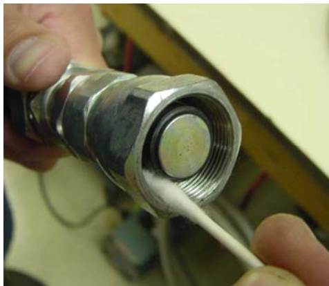
Figure B-1: Cleaning the female Aeroquip
